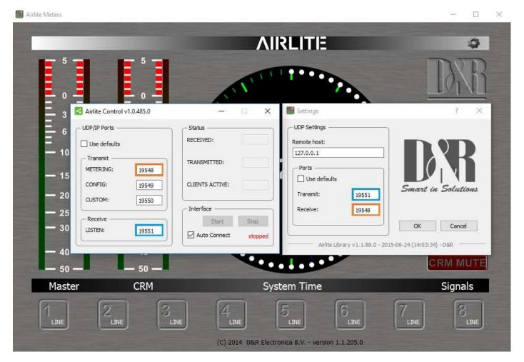
In blue you'll see the port that is used for transmitting the data to control the On switches with the software. (Software to Airlite).
